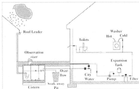
FIGURE 5-15 A Schematic of rainwater harvesting. SOURCE: PaDEP (2006).
